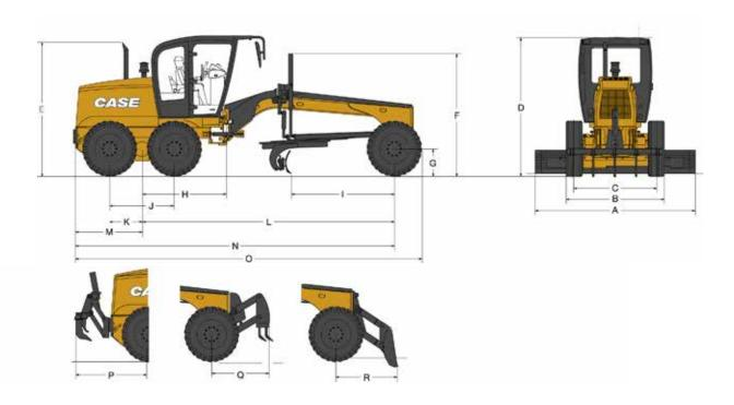
All units fitted with 14.0 x 24-12L tires, open ROPS/FOPS cab, standard battery, full fuel tank, operator weighing 75 kg, specifications in accordance with ISO 7134.
